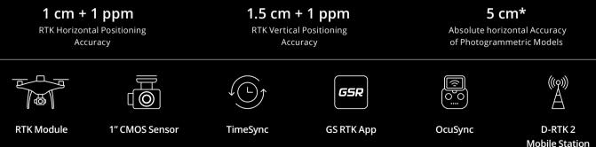
\*when flying in sunny conditions, wind speeds below 4 m/s, 100m height and 2.74 cm GSD, front overlap rate of 80%, side overlap rate of 70%
